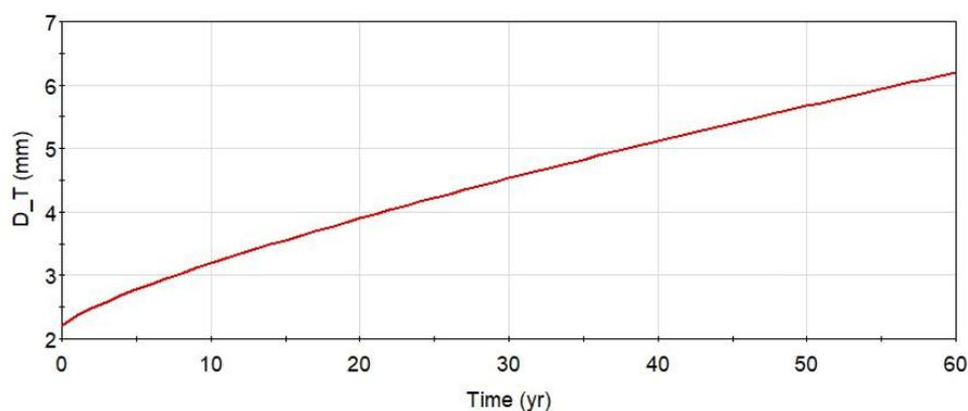
Figure 1. Defects depth growth rate over time forecasted with a power law function.
