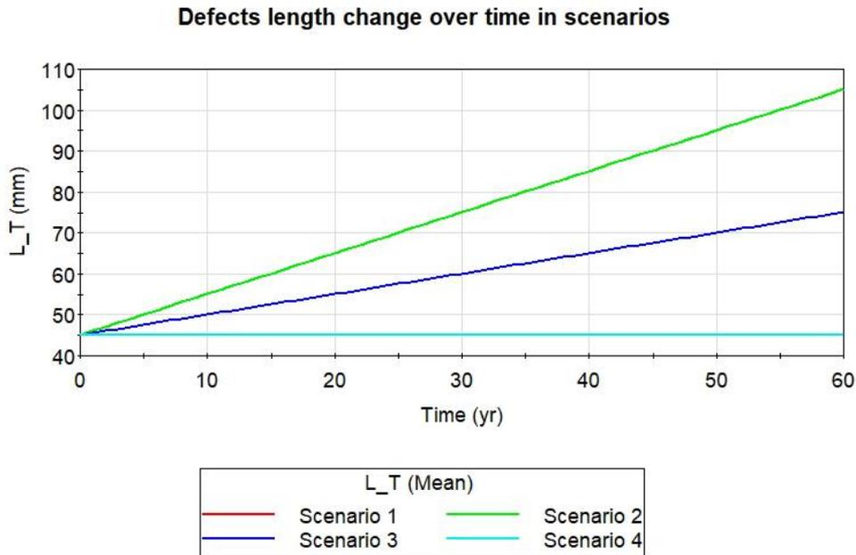
Figure 2a, 2b. Metal losses length growth rates in the axial direction for various scenarios.
