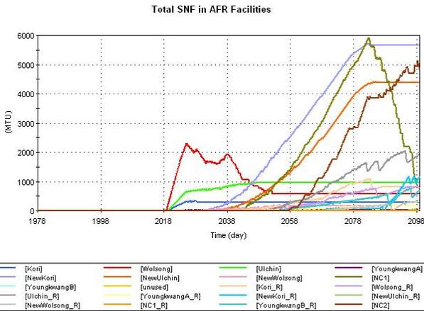
Figure 10. SNF Accumulation at Each ISFSI for the CASE I Study
