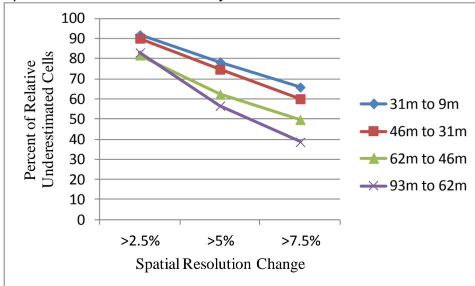
**Figure 12.** Percent of relative underestimated cells for different slope ranges
