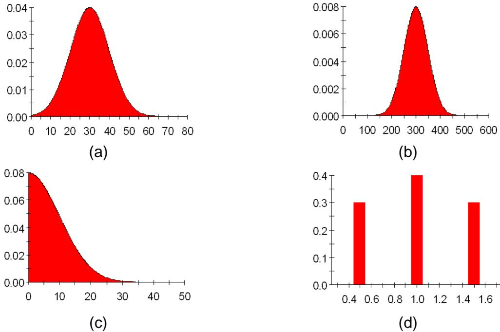
**Figure 2.** Probability distribution curves of: a) time to total failure; b) final bottom width of the breach; c) final elevation of breach bottom; and d) side slope of breach width
