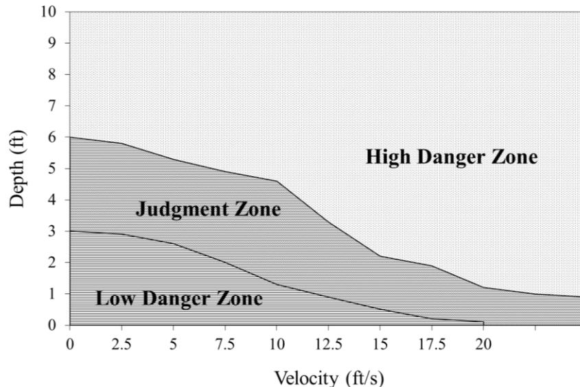
**Figure 3.** Floodwater depth – velocity hazard classification. Source: ACER (1988)
