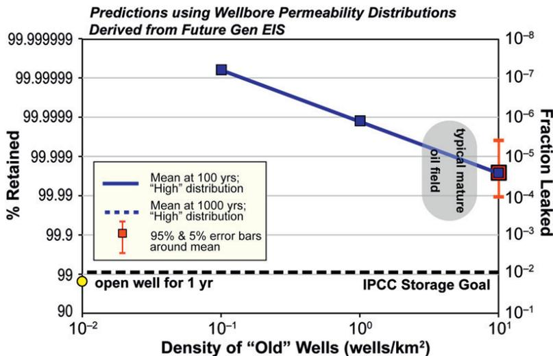
Fig. 3. Effect of wellbore spatial density on amount of CO<sub>2</sub> retained and fraction of CO<sub>2</sub> leaked out of sequestration reservoir.
