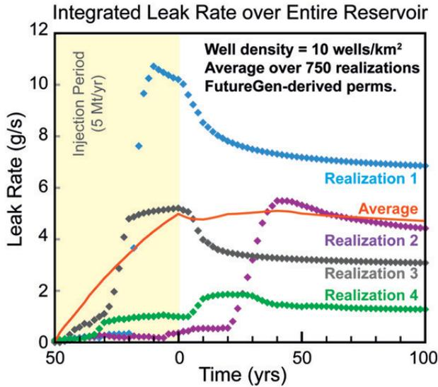
Fig. 2. Example leak rate curves computed using the IAM during a Monte-Carlo calculation.
