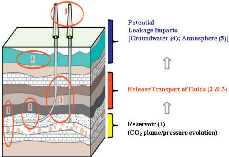
Fig. 1. Sub-systems within IAM structure being developed by NRAP.
