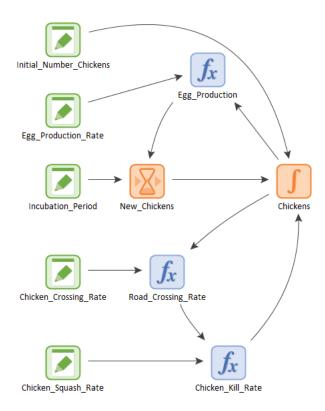
In a sense, GoldSim is like a "visual spreadsheet" allowing you to *visually* create and manipulate data and equations. As can be seen in the simple example shown above, based on how the various objects in your model are related, GoldSim automatically indicates their influences and interdependencies by visually connecting them in an appropriate manner. GoldSim also sets up and solves the equations represented by the objects and their interdependencies.
